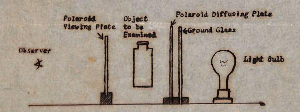
Operation - The glass to be examined is simply placed between the POLROID plates, and tilted through an angle of forty-five degrees. With the Polaroid Plates in the "crossed" position, with their polarizing axes at right angles, practically no light whatever will pass through them from the light source (somewhat less than one-half of one per cent). For this reason the Polaroid Diffusing Plate will appear black.
